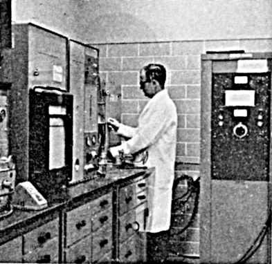
Radiolysis products determined with the x-ray machine (upper left). The radioactivity of a cement mortar sample is checked as it is removed from the thermal neutron irradiation facility (center). Shown below is the drift tube apparatus built for ion-molecule studies.
