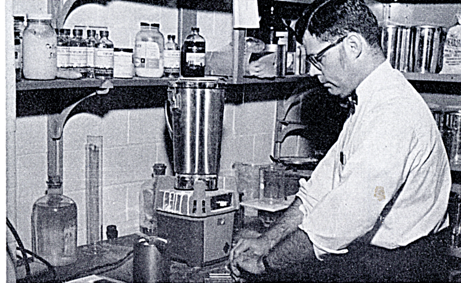
Large scale "blendor" is used in the dispersion of pigments for laboratory paint studies.
