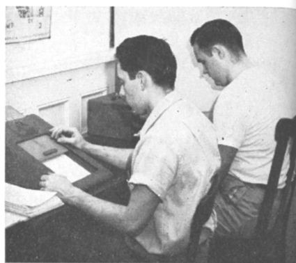
This device employs a shutter that descends over the page at a predetermined rate.
