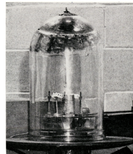
Figure 1. Wires of the metal to be plated by evaporation are hung on the glowing coils above the substrate.
