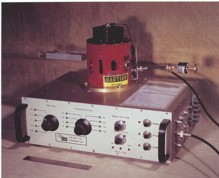
This 95 GHz extended-interaction-amplifier transmitter was developed by GTRI engineers for the U.S. Army
