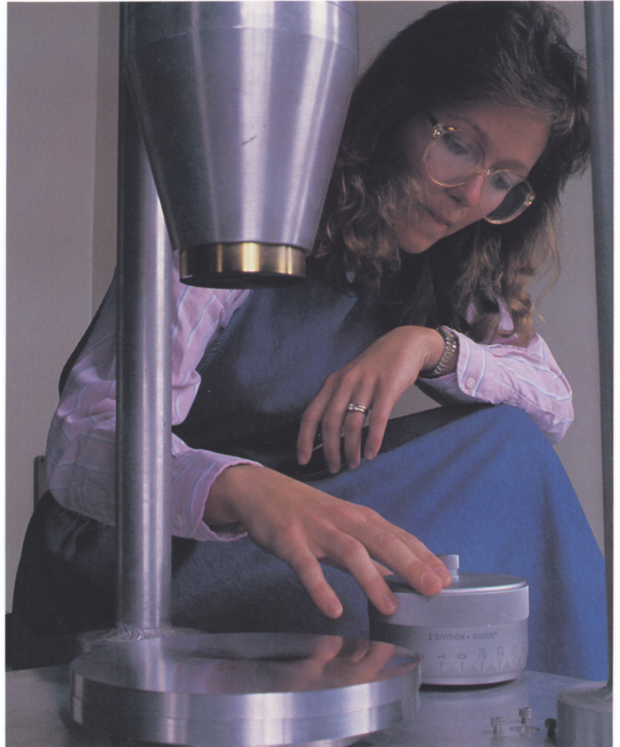
Researchers use this Fabry-Perot interferometer to characterize materials at high millimeter-wave frequencies.
