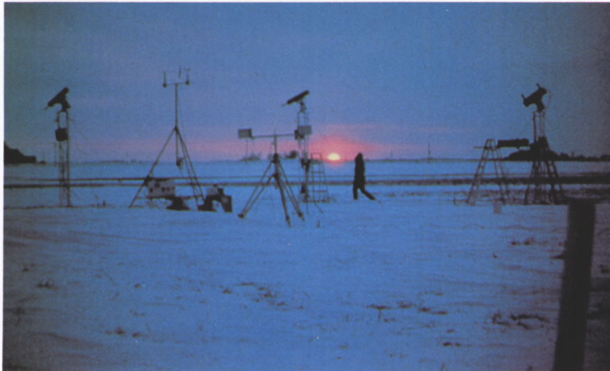
GTRI researchers made a ground-breaking study of millimeter-wave propagation in turbulent atmospheres. Measurements were taken on location at Flatville, Illinois.
