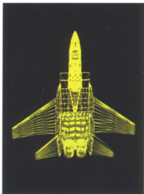
Above: GTRI researchers use a computer model of the F-15 jet aircraft for predicting radar cross section.
