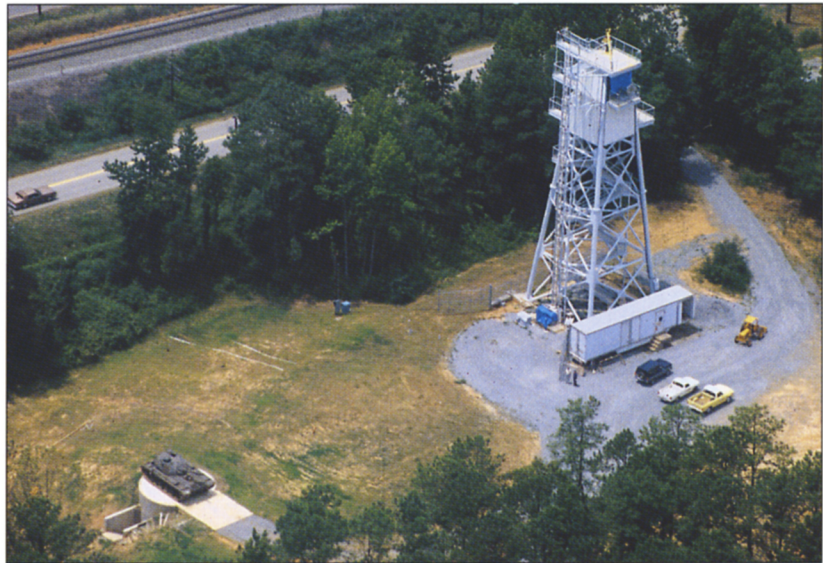
GTRI's Electromagnetic Test Facility, located at the university's Cobb County Research Complex near Dobbins Air Force Base, includes this source tower and radar cross section turntable.
