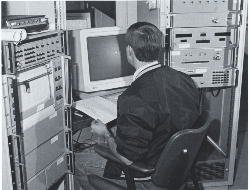
This three-channel programmable microwave receiver is effective from 20 MHz to 107 GHz and uses an assortment of mixers and downconverters.
