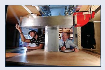
Researcher Robert Englar (right) and co-op student Daniel Hegeman adjust blowing slots on a model truck inverted in GTRI's low-speed wind tunnel. The testing helped assess the value of fuel-saving improvements.
