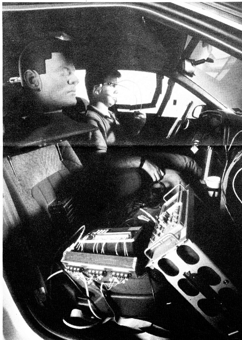
Noise data was collected in a wind tunnel with the car engine off before road tests were begun. (Photo by Gary Meek)
