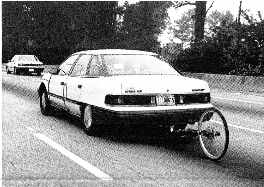
The bicycle wheel attached to the back of the car helped monitor the vehicle's speed. Microphones taped to the car are visible on the left side doors and windows. (Photo by Gary Meek)
