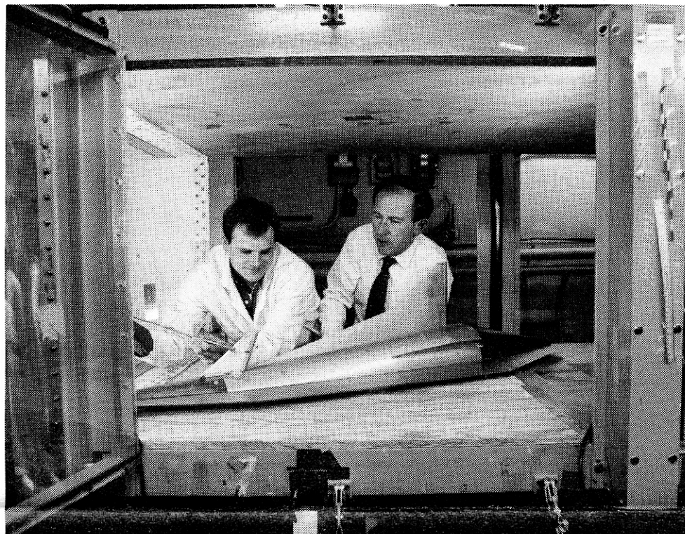
AERO co-op student Kurt Niebur, left, and researcher Bob Englar test the take off and landing aerodynamics of a generic High Speed Civil Transport model for NASA-Langley. They performed the tests during February in the GTRI Model Test Facility research wind tunnel at Cobb County. (Photo by Anita Edwards)
