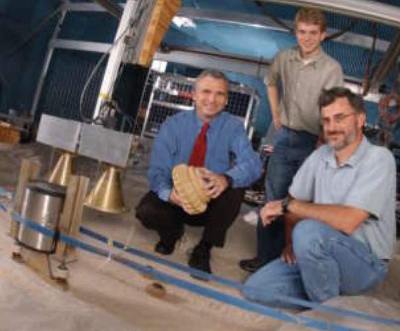
GTRI researchers are working with colleagues at Georgia Tech to develop a land mine detection system that uses high-frequency seismic waves to slightly displace soil and objects in it. A non-contacting radar sensor then measures the results, creating a visual representation that reveals hidden land mines.
