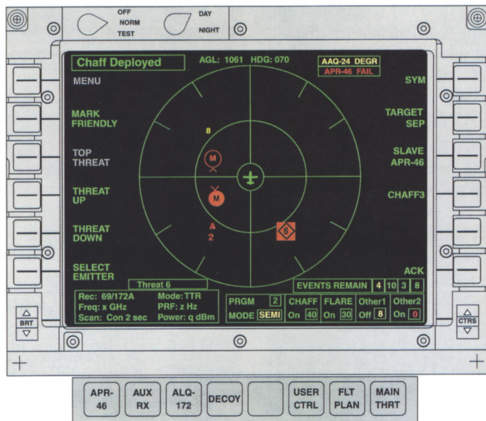
The C-130 Electronic Warfare (EW) Bus System is an integrated electronic countermeasures suite for the C-130 aircraft, with centralized display and control.
