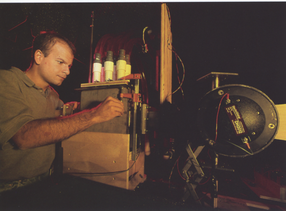
In GTRI's acoustic liner test facility, sound from the black speaker (right) flows through a liner positioned inside a metal box (left).
