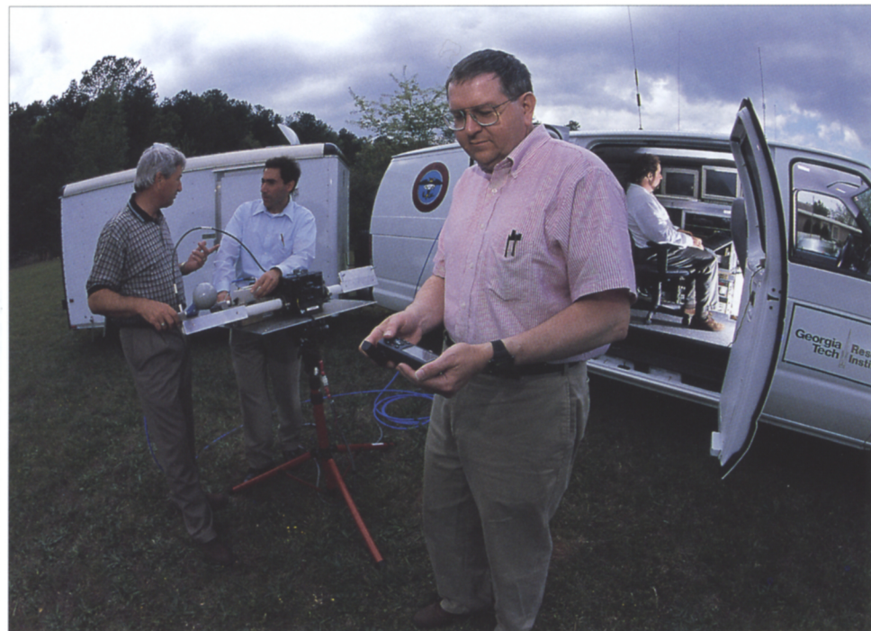
Our Electronic Protection Mobile Test Van allows researchers to test air and ground radars despite challenging field conditions. Here, they adjust equipment that creates false targets.
