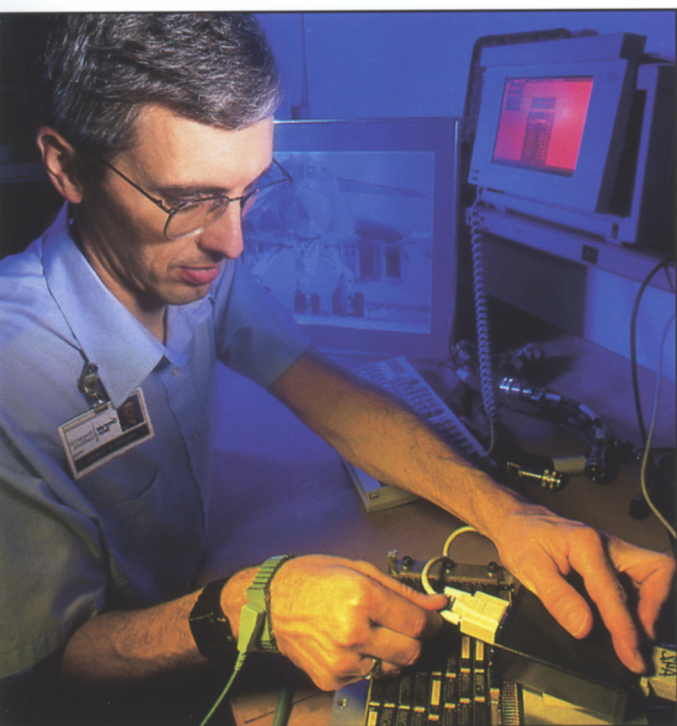
A serial interface unit developed by GTRI allows technicians to reprogram the ALQ-161 system on the flight line using laptop computers.
