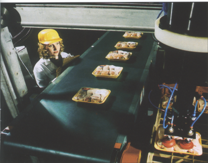
GTRI researchers have developed the Intelligent Integrated Belt Manipulator to help move food packages on the factory floor.
