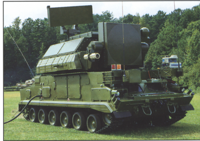
GTRI researchers have developed a mobile radar threat simulator.
