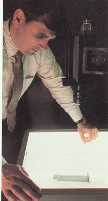
Above, as part of a machine vision development effort, GTRI engineers measure spectral reflectance properties of machine parts. Top right, an integrated optic wave guide used for interferometric sensor studies. Integrated optics shows promise for industrial sensing applications.
