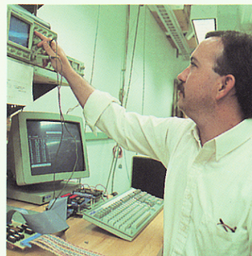
Top left, engineers are continuing to enhance the ALR-69 radar warning receiver, which displays threats on this computer display. Above, GTRI has developed engineering support stations for controlling and collecting data from the ALR-69.
