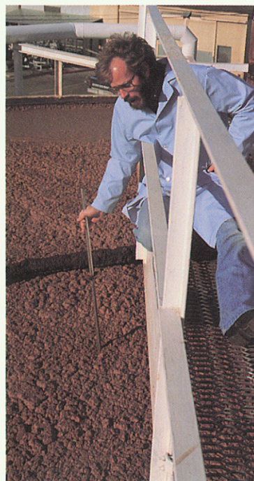
Top left, GTRI researchers helped install computers in poultry growout houses. Near left, a Thermally Enhanced Dewatering System was developed at GTRI for recycling nutrients in poultry processing plant wastewater.
