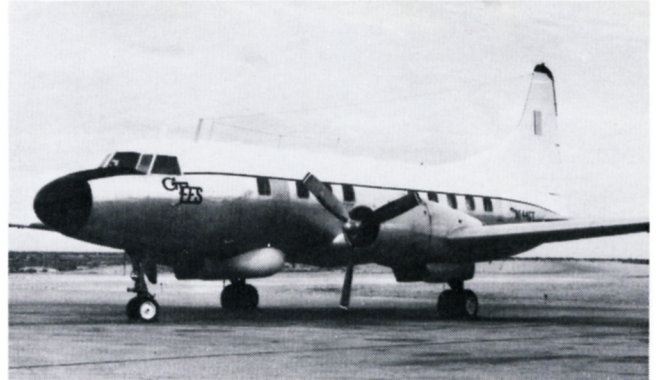
The EES airborne electronics laboratory, used for flight tests of experimental ECM equipment, also is available for atmospheric sampling.
