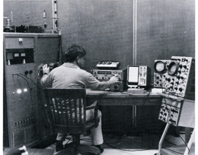
High-power source for electromagnetic measurements used in testing cardiac pacemakers.
