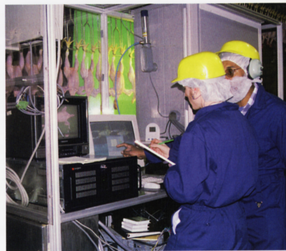
An automated computer vision system being developed at GTRI could detect defective chickens and signal removal of them from processing lines.
