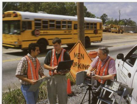
*The Safety Warning System developed at GTRI sounds an alarm and displays advisory text messages on an LED screen in vehicles as they enter work zones or other caution areas.*
