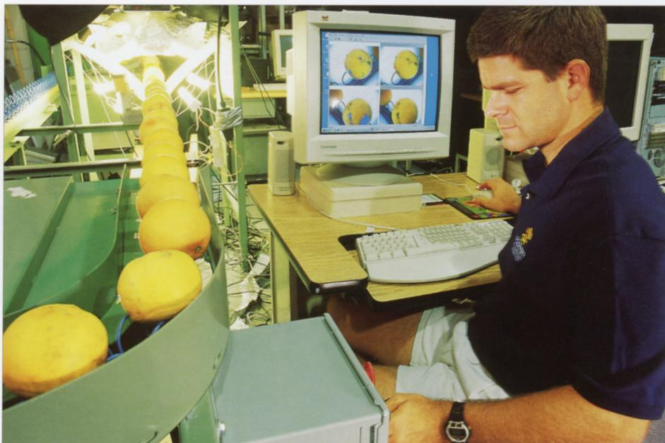
*To image and grade 600 grapefruit per minute, GTRI developed computer algorithms that are executed on a 500-MHz Pentium processor in about 10 milliseconds.*
