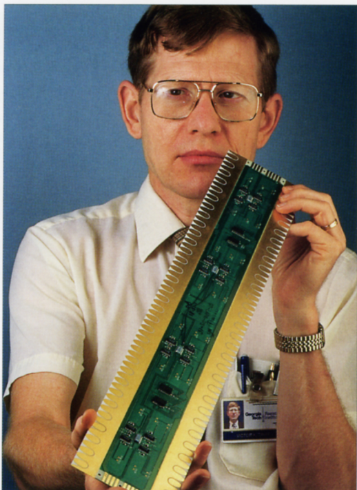
This aperture printed circuit board is the fundamental lens building block for the lightweight airborne phased-array radar antenna.
