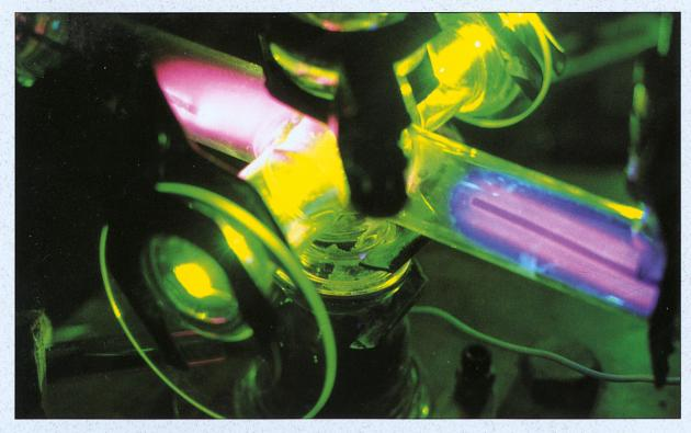
GTRI scientists developed a novel laser-induced fluorescence technique to optically detect silicon atoms and silicon monoxide molecules.
