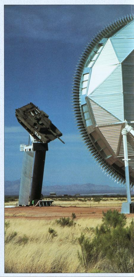
limeter-wave antennas mounted on full-size aircraft, tanks, and other vehicles. The system includes an offset-fed parabolic reflector 75 feet in diameter, a novel positioner capable of supporting up to 70 tons, and a set of five feedhorns to cover frequencies from 6 to 40 GHz.
