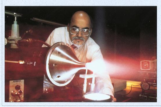
properly inserted in the exhaust nozzle, the tabs aid in the rapid mixing of plume gases with air flowing past the aircraft.
