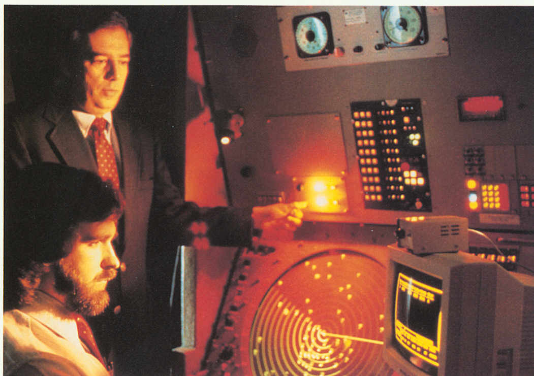
■ ■ GTRI engineers built a computer-based system that automatically monitors radar returns, alerting the human operator only when a potential target is detected.
