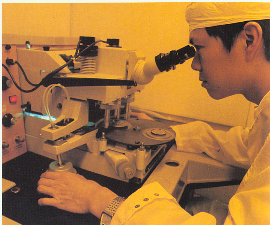
■ ■ Above, GTRI scientists used modern photolithographic techniques to fabricate miniaturized optical waveguide circuits for potential use as optical switches.
