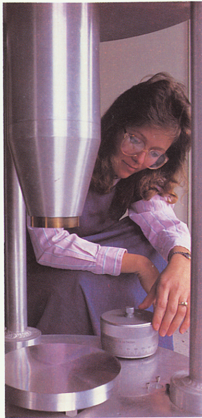
■ ■ Above, researchers use this Fabry-Perot interferometer to characterize materials at high millimeter wave frequencies.
