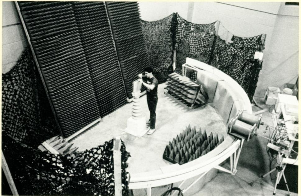
conducted infrared and millimeter wave measurements as part of the Defense Department effort to evaluate and eventually develop dual-mode seekers.
