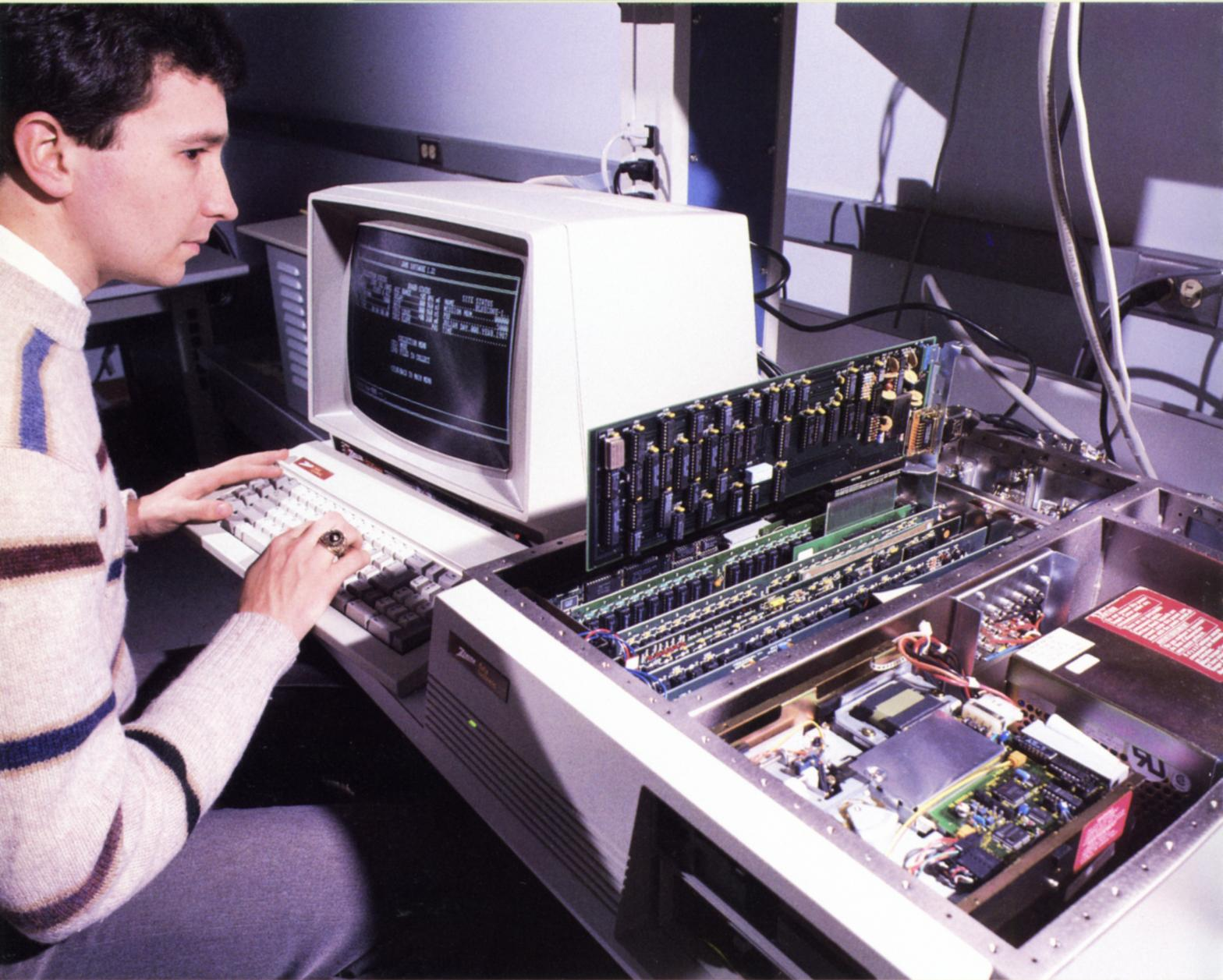
*Above, researchers here developed this radar data acquisition system to quantify radar and electronic countermeasures signals in a flight test environment at Eglin AFB. Right, research continued on a laboratory prototype which delivers localized auditory cues to a pilot through earphones.*
