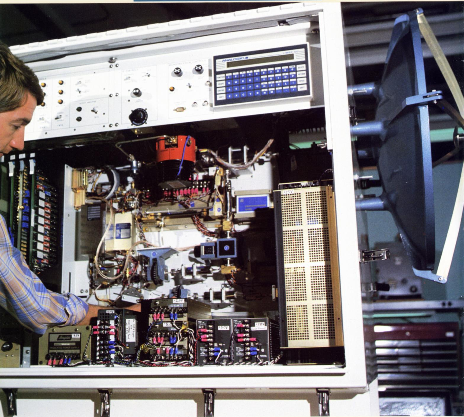
*Above*, engineers completed development of HIIPCOR, the first high-power, coherent radar system operating at 95 GHz. *Far right*, this 90-foot source tower is part of a large Electromagnetic Test Facility which became fully operational during the past fiscal year.
