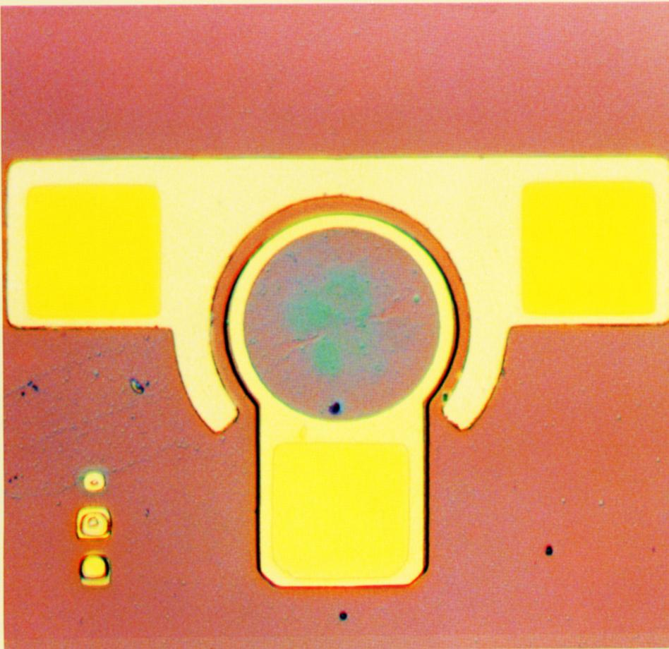
**Last year, Tech researchers used molecular beam epitaxy to grow optoelectronic devices of high purity such as this gallium arsenide pin avalanche photodiode. The device is 150 microns in diameter.**
