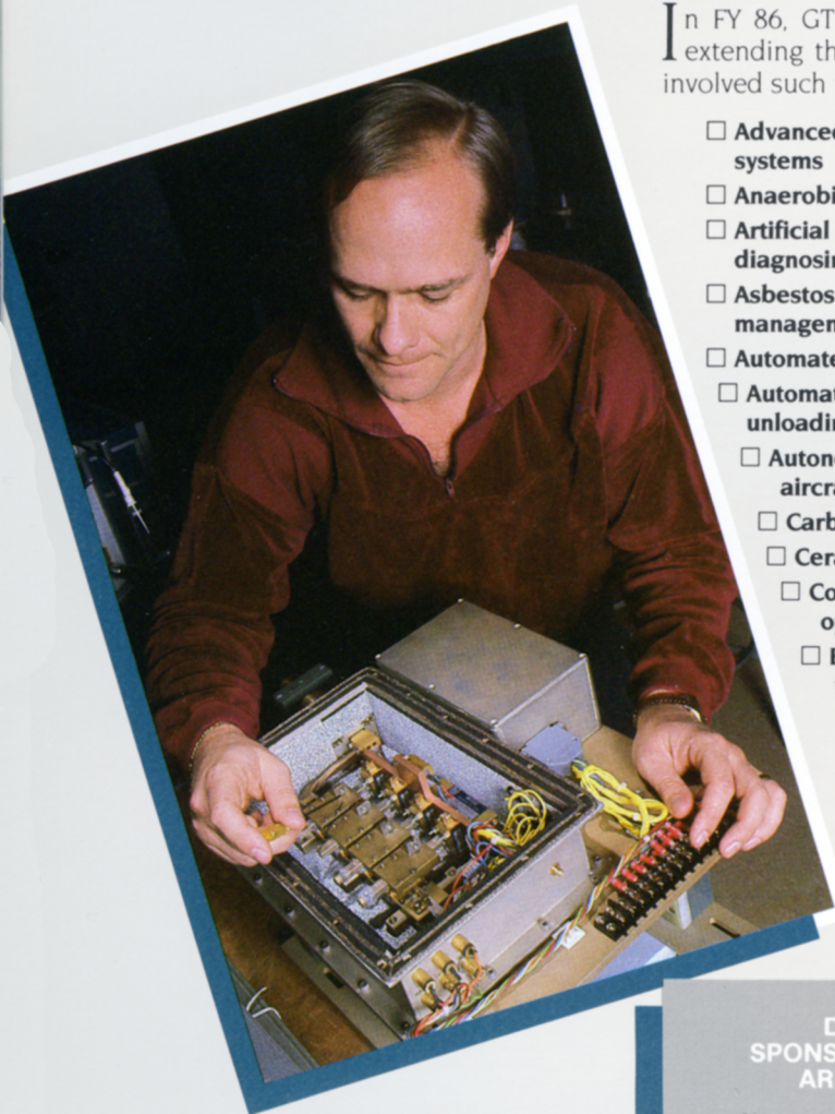
Above, this 30-40 GHz receiver is part of a tactical millimeter wave direction finding system developed for the U.S. Army. Facing page, GTRI's Electromagnetic Test Facility is a state-of-the-art complex for precision antenna measurements, radar cross section measurements, electronic system measurements, and propagation studies.
