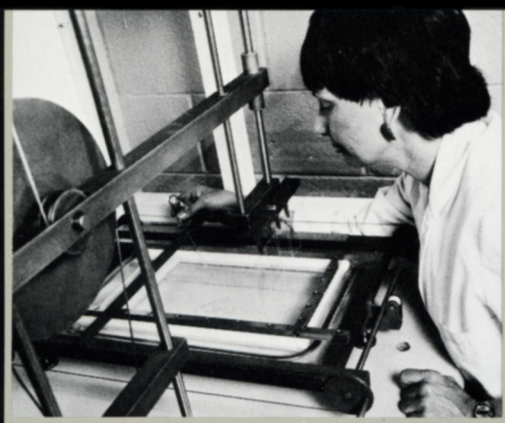
The Station is capable of constructing oriented monomolecular assemblies with a Langmuir-Blodgett trough.
