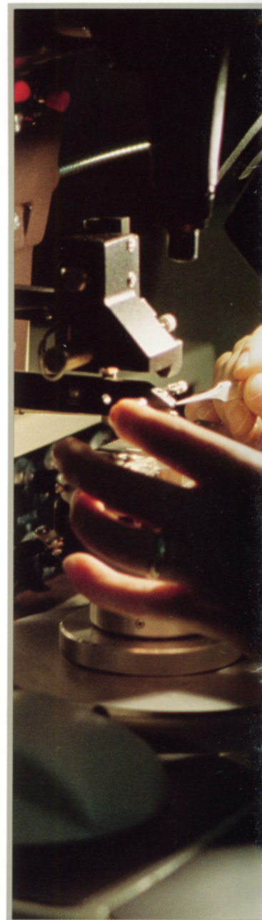
EES makes wire bonds which electrically connect integrated circuits to package leads.
