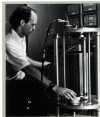
This five band Fabry-Perot interferometer is used for measurements of complex permittivity and permeability of materials.
