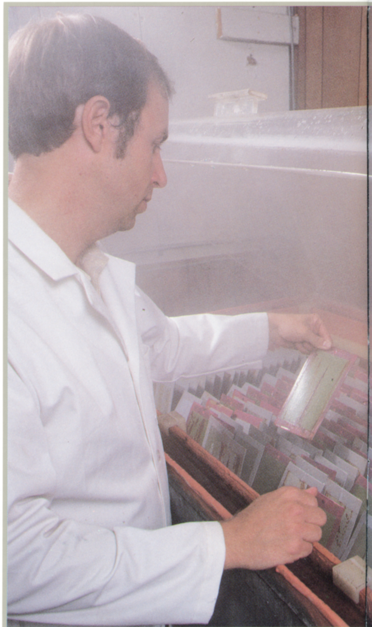
This salt fog cabinet accommodates tests of paints and coatings intended to protect steel from corrosion.
