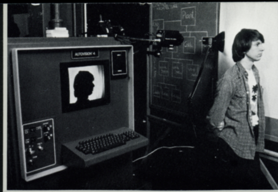
EES engineers use this vision system to process tactile sensing information.
