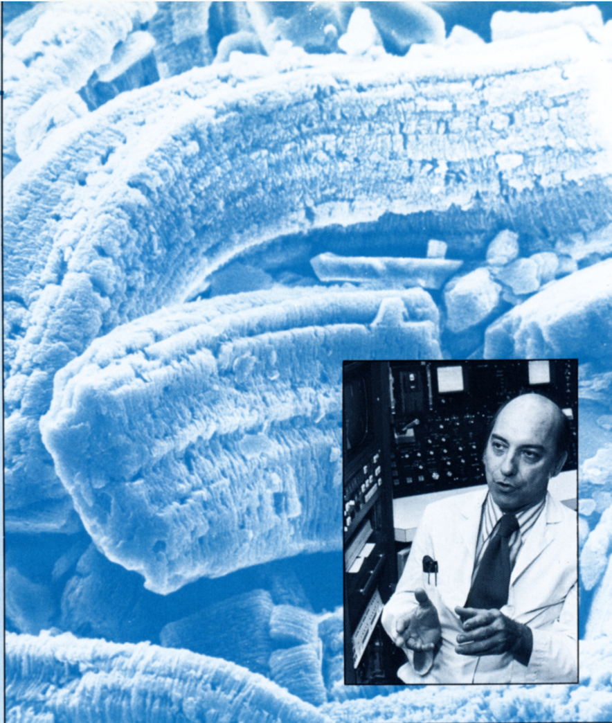
John Brown (above) explains how this scanning electron microscope is used by EES to determine why materials fail to function in specific applications. These kaolin clay particles were magnified 2,000 times to evaluate the chemical characteristics of clay taken from 120 sites in Georgia.
