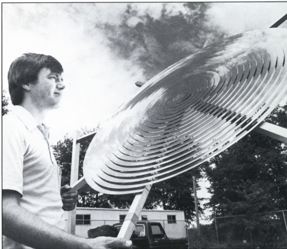
EES engineer Rick Steenblik (above) designed this solar concentrator which can generate temperatures of 2000°F.
