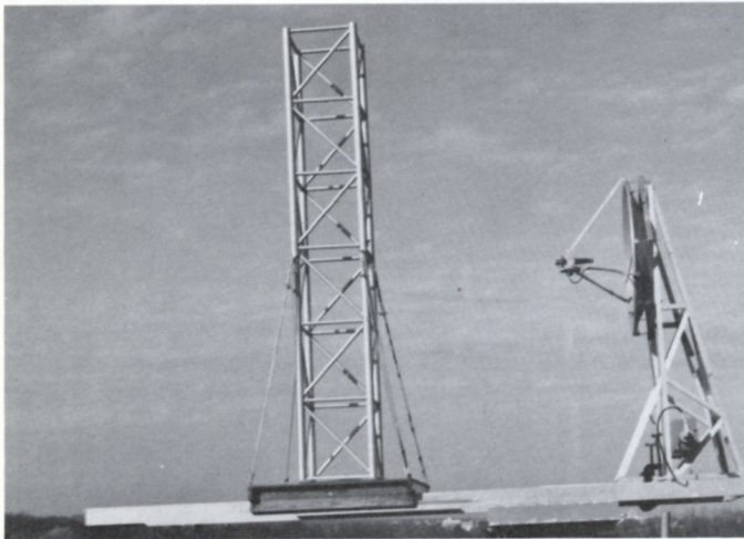
Measurements being performed on a monopulse antenna and obstacle combination to determine effects of a near-field obstacle on the tracking accuracy and gain loss of the antenna.
